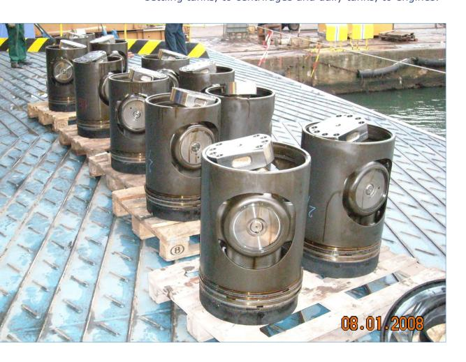
On January 8, 2008, after fifteen months of continuous operation with **XBEE** HFO, the ship entered the Remontowa shipyards in Gdansk, Poland, for her first service after thirty thousand hours of work.
